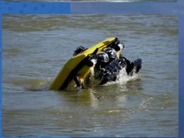
"The TRV series has sufficient thrust to allow proven operations in currents up to 4 knots and down to depths of 3,300'..."
